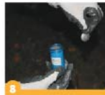
8 Take the igniter powder and metal plate from inside of the box.
